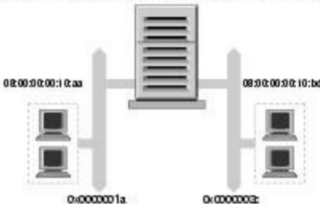
A file server attached to two IPX networks with an internal network.
