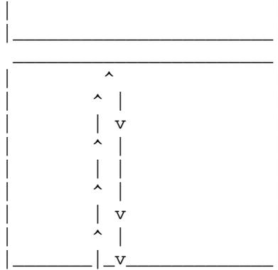
The vertical sync frequency is the number of times per second that the monitor's electron beam can trace a pattern like this
