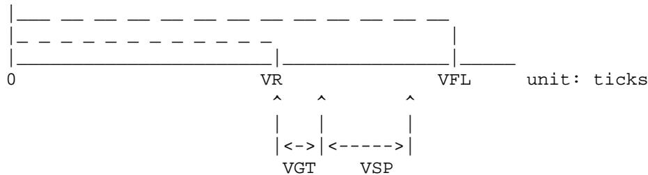
We start the sync pulse just past the end of the vertical display data ticks. VGT is the vertical guard time required for the sync pulse. Most monitors are comfortable with a VGT of 0 (no guard time) and we'll use that in this example. A few need two or three ticks of guard time, and it usually doesn't hurt to add that.
