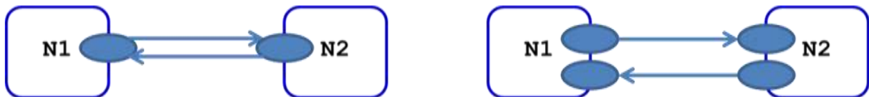
Figure 2a. Bi-directional TE link combination (left), independent uni-directional TE links (right)
