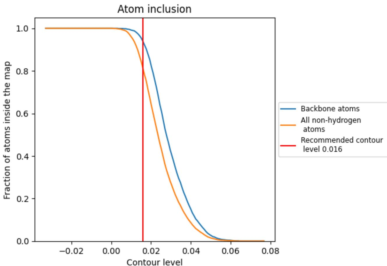
At the recommended contour level, 94% of all backbone atoms, 81% of all non-hydrogen atoms, are inside the map.
